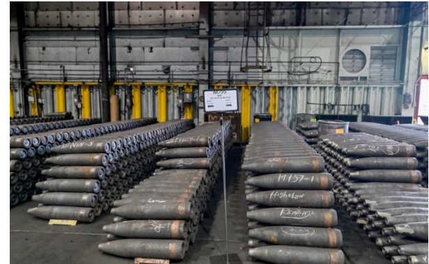
Rows of incomplete 155mm shells wait for the next step in production at the Scranton Army Ammunition Plant (Photo by Aimee Dilger/SOPA Images/Light Rocket via Getty Images)
